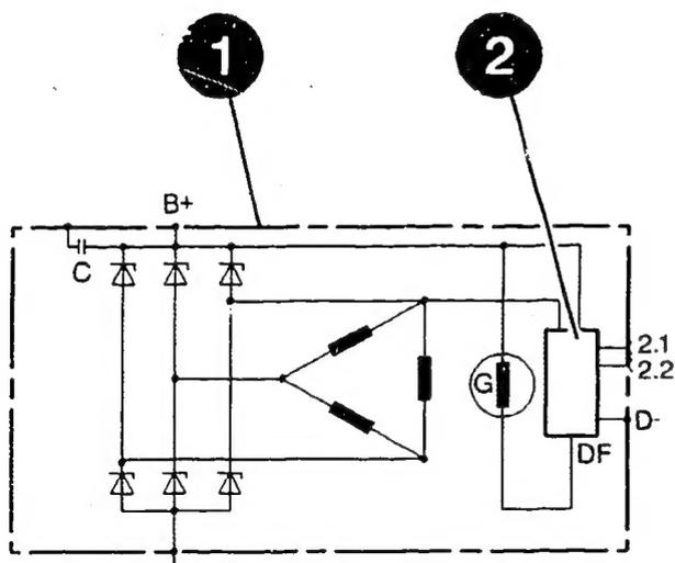
The NF alternator was fitted for the first time as of 6/98 in the BMW 540i (E 39) and 740i (E 38) with engine M62 (8-cyl.).
